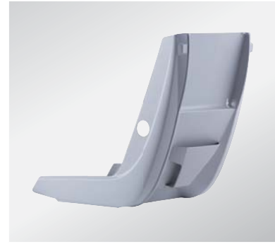
Rail seat bucket, made from flame-resistant plastic, mounted from several parts
