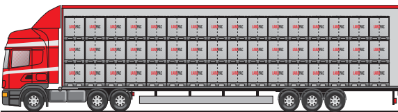
Hintransport (Mega-Trailer / Jumbo): 96 vollbeladene LARAPAC-Systeme (1200 x 800)
